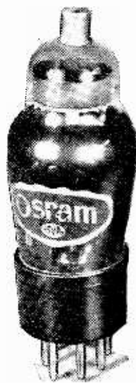
Osram KTZ41 television RF pentode with mutual conductance of 12 mA/V.
